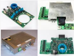
Digital gate units
