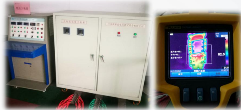
Temperature rise test: low voltage high current equipment, thermal imager
